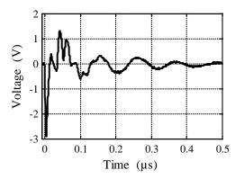
Fig. 8. Voltage measurement inside the stator.
