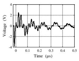
Fig. 6. Voltage pulse measurement on the cable.
