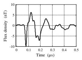
Fig. 9. Flux density due to the partial discharge measured in the cooling gap between the stator core and the frame.
