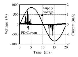
Fig. 5. Partial discharge current (AC-50 Hz).
