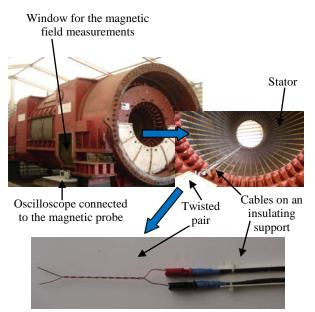
Fig. 3. An instrumented 125 MW stator available in LSEE.
