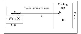
Fig. 2. Magnetic field due to PD between two stator bars.
