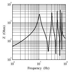
Fig. 11. Frequency analysis of the equivalent impedance of the cable.
