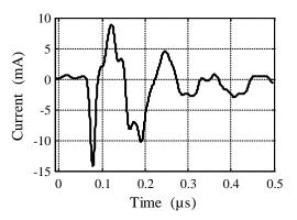
Fig. 10. Partial discharge current in the cable.
