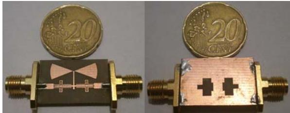
Fig. 8. The photograph of the fabricated UWB BPF.
