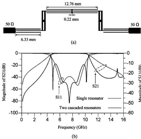
Fig. 5. Two cascaded resonators: (a) schematic, and (b) simulation.
