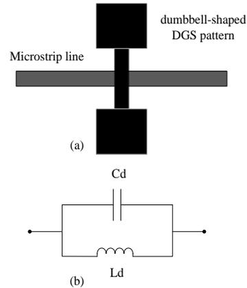
Fig. 6. DS-DGS: (a) layout, and (b) LC model.
