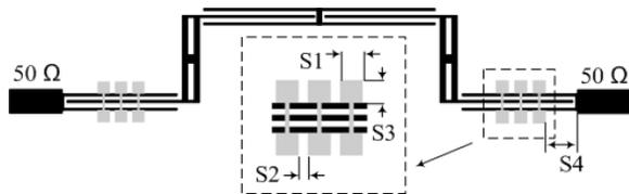
Fig. 8. Layout of the final filter.
