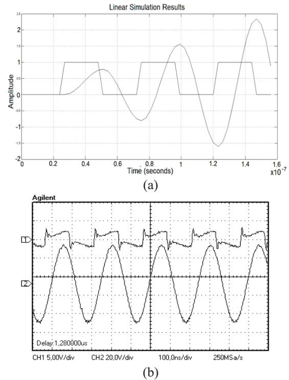
Fig. 6. Resonance of Tesla coil; frequency of square wave approximately equal to frequency of step response: (a) simulated response for transient response (sum of responses), and (b) experimental result.
