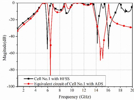
Fig. 5. Transmission magnitude of the unit-cell No.1 obtained by HFSS and by equivalent circuit model ( $C_{S1}=0.033$  pF;  $L_{S1}=18.42$  nH;  $C_{S2}=0.036$  pF;  $L_{S2}=2.92$  nH;  $C_{P1}=0.22$  pF;  $L_{P1}=1.595$  nH;  $C_{P2}=0.064$  pF;  $L_{P2}=4.52$  nH, coupling coefficient  $k_1=0.14$ ,  $k_2=0.14$ ).
