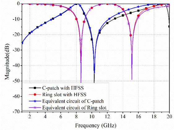
Fig. 4. Reflection magnitude of the C-patch and ring slot of the unit-cell No.1 in free space, obtained by HFSS and by equivalent circuit model ( $C_{S1}=0.021$  pF;  $L_{S1}=18.42$  nH;  $C_{S2}=0.024$  pF;  $L_{S2}=2.92$  nH;  $C_{P1}=0.135$  pF;  $L_{P1}=1.595$  nH;  $C_{P2}=0.039$  pF;  $L_{P2}=4.52$  nH).
