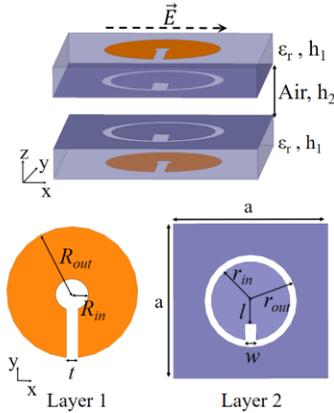
Fig. 1. Geometry of the proposed transmitarray unit-cell structure.
