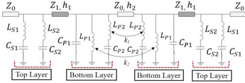
Fig. 3. Equivalent circuit model of our proposed unit-cell.
