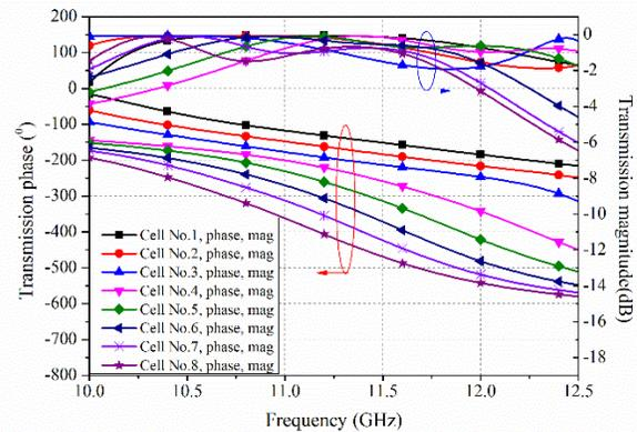
Fig. 2. Simulated transmission coefficients of eight unit-cells.
