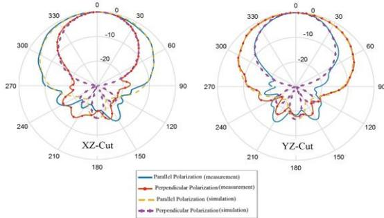
Fig. 11. Normalized radiation pattern in linear polarization mode.
