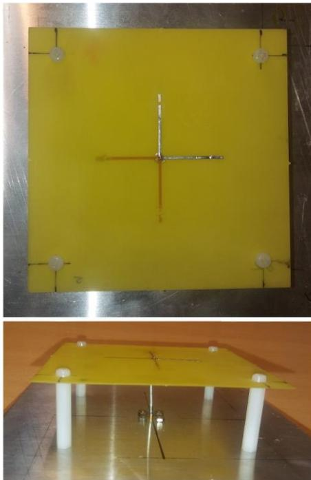
Fig. 8. Photos of RHCP crossed dipole antenna.
