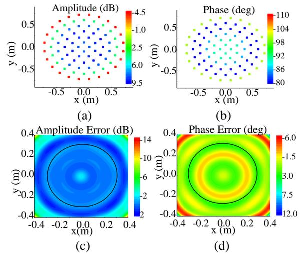
Fig. 6. Simulation results of the PWG based on the sub-array method at 3 GHz. The amplitude (a) and phase (b) of the excitations of the antenna elements in the PWG; the amplitude (c) and phase error (d) on the AUT.
