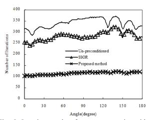
Fig. 5. Iterative number for an open cavity with unpreconditioned GMRES method, SSOR preconditioner, and the proposed method.
