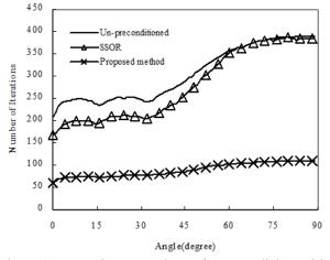
Fig. 6. Iterative number for a disk with unpreconditioned GMRES method, SSOR preconditioner, and the proposed method.
