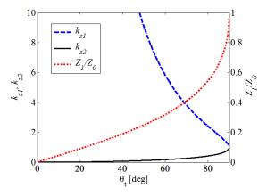
Fig. 2. Impedance ratio  $(k_{z1} \text{ and } k_{z2})$  and normalized impedance  $Z_1$  versus total electrical length of SITL,  $\theta_t$ .
