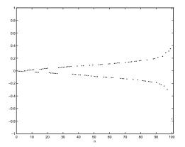
Figure 2: Plot of the smaller normalized eigenvalues for the  $TM_z$  scattering from a circular cylinder of radius  $a=\frac{\lambda}{2}$  (Problem Size 128 × 128).
