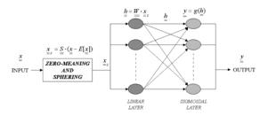
Figure 1- Architecture of the Infomax Neural Network
