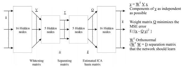
Fig. 2- The Neural Network feed-forward scheme for computing ICA.
