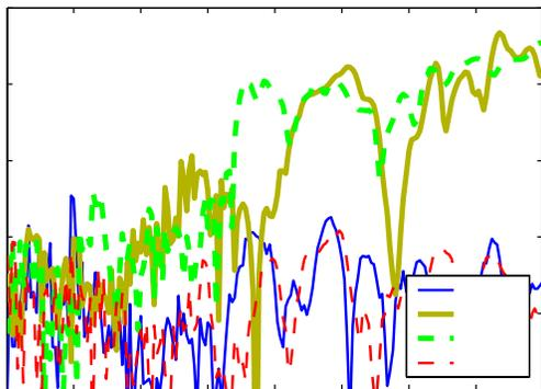
Figure 5d. Measured net transmission between two horizontal halfwave dipoles located 9mm above the 4 different surfaces.
