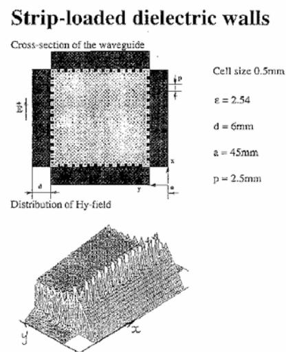
Figure 3b. Geometry (upper) and computed H-field distribution (lower) in dual-polarized quasi-TEM hard waveguide realized by modeling each metal strip of finite thickness. The computations have been done by FDTD as explained in [16].
