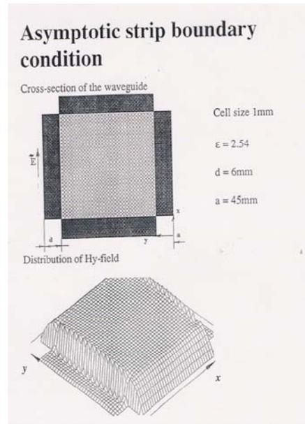
Figure 3a. Geometry (upper) and computed H-field distribution (lower) in dual-polarized quasi-TEM hard waveguide realized by strip-loaded dielectric substrate. This case has been computed by using the asymptotic strip boundary condition [17].
