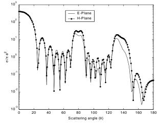
Fig. 5: Normalized bistatic cross-section patterns for eight identical dielectric spheres each covered with a dielectric layer with ka=2.0, kb=2.5, kd=7.0,  $\alpha = 0, \mathcal{E}_{Ir} = 3.0$ , and  $\mathcal{E}_{IIr} = 2.0$ .
