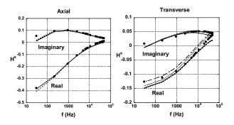
Figure 6. Comparison of the measured EMI signal from the fragment in Figure 5 (lines) with that calculated for a prolate spheroid with a = 1.25 cm, b = 5 cm,  $\sigma = 2.6 \times 10^6$  (S/m),  $\mu = 36\mu_0$  (dots). Different line types are for measurements from different views (i.e. up and down for the axial case, and four 90° rotations about the axis for the transverse case).
