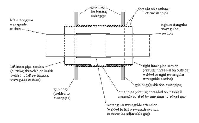
Figure 5. Schematic Diagram of Adjustable Length Rectangular Waveguide
