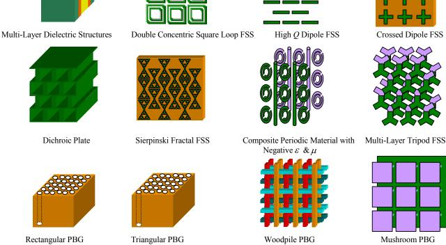
Fig. 2: Different classes of complex EBG structures characterized by the FDTD/Prony/ARMA technique.
