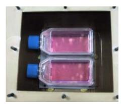
Figure 3. Two culture flasks, each filled with 6 mm of RPMI, placed in the middle of the top half of the TEM cell.
