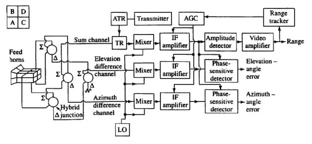
Figure 2. Schematic Diagram of Two-Coordinate (Azimuth and Elevation) Amplitude-Comparison Monopulse Tracking
