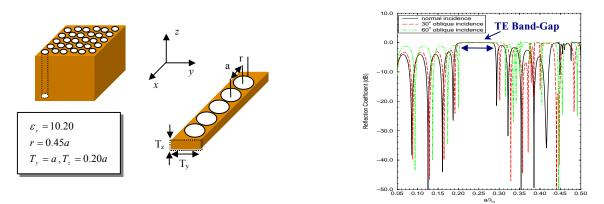
Fig.6: 5-Layer rectangular PBG, (a) Periodic structure, (b) Normal and oblique incidence reflection coefficient.
