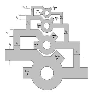
H-plane dimensions  $a_0^{>} a_1^{>} a_2^{>} a_3^{-}$  for the parallel (P), summing arms of the hybrid junctions. Some E-plane dimensions for the series (3), difference arms of the hybrid junctions may be equal, depending on the mode selected.
