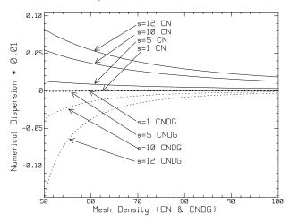
Fig. 3 Numerical anisotropy for CN and CNDG.
