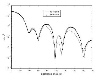
Fig. 3: Normalized bistatic cross section patterns for three identical dielectric spheres each covered with dielectric layer with ka=2.0, kb=2.5, kd=7.0,  $\alpha = 0, \mathcal{E}_{Ir} = 3.0$ , and  $\mathcal{E}_{IIr} = 2.0$ .
