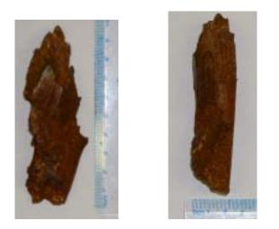
Figure 5. Piece of ordnance scrap on which measurements were performed, with length about 10 cm, width in one transverse direction 3~4 cm and about 2cm in the other.
