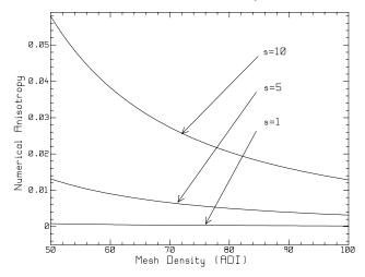
Fig. 2 Numerical anisotropy of the ADI method at Courant numbers 1,5 and 10.
