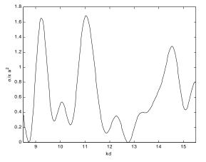
Fig. 6: Normalized backscattering cross section versus electrical separation (kd) for end-fire incidence and a linear array of five identical dielectric spheres each covered with a dielectric layer with: ka=4.0, kb=3.0,  $\alpha = 0.0$ ,  $\mathcal{E}_{Ir} = 3.0$ , and  $\mathcal{E}_{IIr} = 2.0$ .
