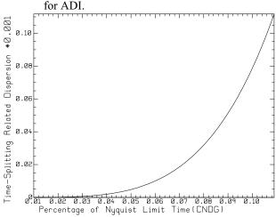
Fig. 7 Intrinsic temporal anisotropy with zero mesh size for CNDG.
