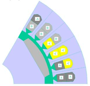
Fig. (1) One pole of the 2-hp Motor
