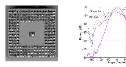
Fig. 11: Enhanced performance microstrip antenna with EBG around: (a) a photo of the design and (b) measured radiation patterns of various microstrip antenna designs. It is noticed that the microstrip antenna with EBG around has the highest gain and lowest back lobe.
