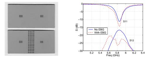
Fig. 12: Microstrip antenna array with reduced mutual coupling: (a) photos of microstrip antenna arrays with and without EBG in between and (b) measured return loss and mutual coupling results of the arrays. It is observed that the mutual coupling is greatly reduced when the EBG is inserted between patch elements.
