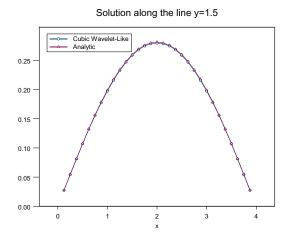
Fig. 18. Numerical and analytic solution along the line y=1.5.
