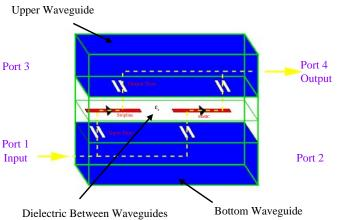
Fig. 1. Aperture-coupled stripline-to-waveguide transition.
