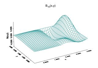
Fig. 14. Cubic wavelet-like basis function obtained from a  $2^{nd}$  level x and  $1^{st}$  level y function.
