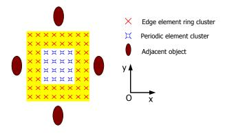
Fig. 3: Schematic of a Hybrid Edge-Periodic DSR model for the analysis of an LPA in the vicinity of other objects.
