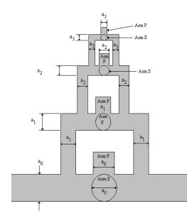
Diameters  $a_0^> a_1^> a_2^> a_3^>$  provide selection of successively higher modes in a manner similar to cascading high-pass filters with successively higher cut-off frequencies.
