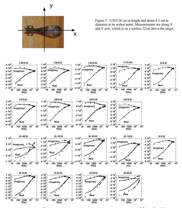
Figure 8. Scattered field  $H_z$  (in ppm) of UXO (markers) and its representative spheroid (a = 2.2 cm, b = 14 cm) along X and Y axis.  $\sigma = 4 \times 10^6$ ,  $\mu_r = 227$ ,  $x_0 = 3.8 cm$ ,  $y_0 = -0.93 cm$ ,  $z_0 = -22 cm$ ,  $\phi_0 = 0$ ,  $\theta_0 = \pi/2$ .
