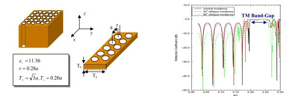
Fig.7: 5-Layer triangular PBG, (a) Periodic structure, (b) Normal and oblique incidence reflection coefficient.
