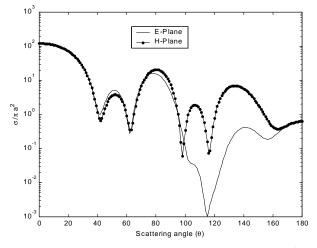
Fig. 2: Normalized bistatic cross section patterns for three identical dielectric spheres each covered with dielectric layer with ka=2.0, kb=2.5, kd=7.0,  $\alpha = 0, \varepsilon_{Ir} = 3.0$ , and  $\varepsilon_{IIr} = 1.0$ . In the E-plane ( $\phi = \pi/2$ ) and H-plane ( $\phi = 0$ ).
