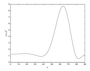
Fig. 8: Normalized backscattering cross section versus aspect angle  $\alpha$  for a linear array of three identical dielectric spheres each covered with a dielectric layer with ka=1.5, kb=1.0, kd=3.0,  $\mathcal{E}_{Ir}$  =4.0, and  $\mathcal{E}_{IIr}$  =3.0.
