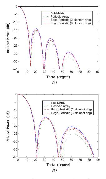
Fig. 4: Far-field radiation patterns of a uniform 8x8element array of microstrip dipoles etched on a foam substrate ( $\varepsilon_r$ =1.03) of thickness 0.19 $\lambda_o$ : (a) E-plane, and (b) H-plane. Dipole lengths and widths are 0.39 $\lambda_o$  and 0.002 $\lambda_o$ , respectively, and element spacings in the x- and ydirections are 0.5 $\lambda_o$  and 0.333 $\lambda_o$ , respectively.
