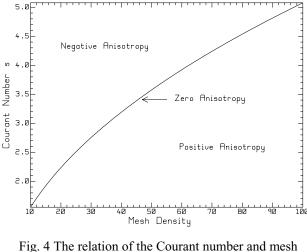
Fig. 4 The relation of the Courant number and mesh density at zero anisotropy for CNDG.
