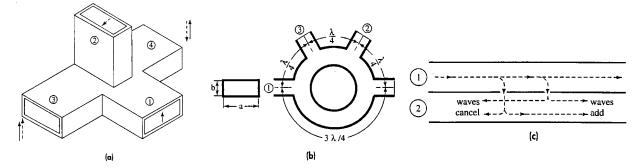
Figure 1. Schematic Diagram of Four-Port Hybrid Junctions. (a) Magic Tee (b) Hybrid Ring (c) Directional Coupler
