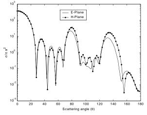
Fig. 4: Normalized bistatic cross section patterns for five identical dielectric spheres each covered with a dielectric layer with ka=2.0, kb=2.5, kd=7.0,  $\alpha = 0, \mathcal{E}_{Ir} = 3.0$ , and  $\mathcal{E}_{IIr} = 2$ .
