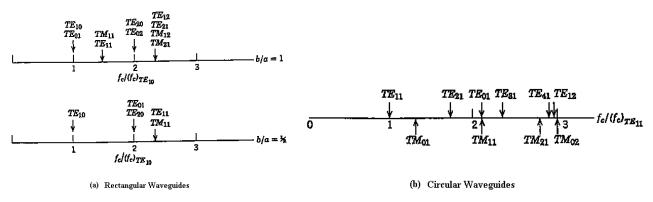
Figure 4. Relative Cutoff Frequencies of Higher Order Modes in Waveguides
