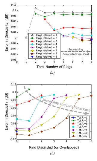
Fig. 8: Hybrid Edge-Periodic cost function curves for a non-uniform 24x24-element array: (a) effect of increasing number of rings retained, and (b) effect of overlapping regions, represented as rings discarded (where Tot.R. = Total Rings), for a particular total number of rings. All other array parameters are the same as in Fig. 5.
