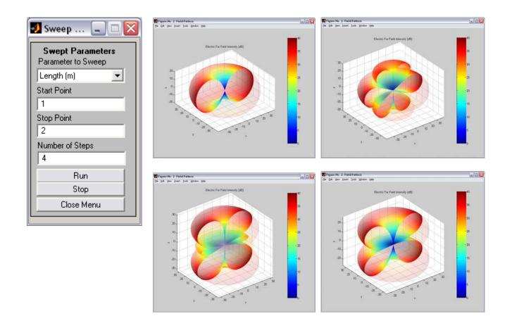
Figure 3. Sweeping a dipole from L=1m to 2m ( $\lambda$ =1m).
