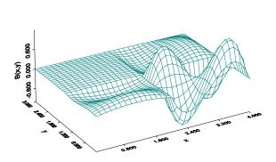
Fig. 15. Cubic wavelet-like basis function obtained from a  $2^{nd}$  level x and  $2^{nd}$  level y function.
