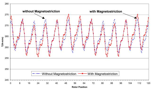
Fig. (6) Torque pulsation with and without Magnetostriction effect.
