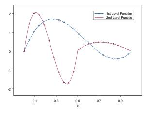
Fig. 9. Third order wavelet-like basis functions from the 1<sup>st</sup> and 2<sup>nd</sup> levels.
