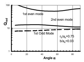
Fig.4: Radiation Quality factor of the first two even modes and the first odd mode.
