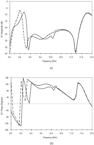
Fig. 9. MoM (solid line) and HFSS (dashed line) comparison of  $S_{11}$  for the  $1 \times 2$  one lower slot, one strip, and one upper slot waveguide coupler array. (a) Magnitude and (b) phase.
