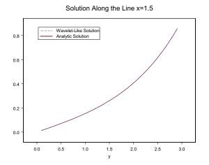
Fig. 17. Numerical (with 961 linear 2D wavelet-like basis) and analytic solutions along the line x = 1.5.
