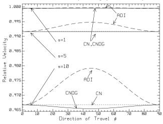
Fig. 1 Numerical dispersion with mesh density 100 and s=1, 5 and 10, for ADI, CN and CNDG.
