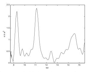
Fig. 7: Normalized backscattering cross section versus electrical separation (kd) for end-fire incidence and a linear array of eight identical dielectric spheres each covered with a dielectric layer with: ka=4.0, kb=3.0,  $\alpha = 0.0$ ,  $\varepsilon_{Ir} = 3.0$ , and  $\varepsilon_{IIr} = 2.0$ .
