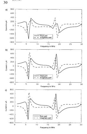
Fig. 2. Complex current induced in a wire loop.
