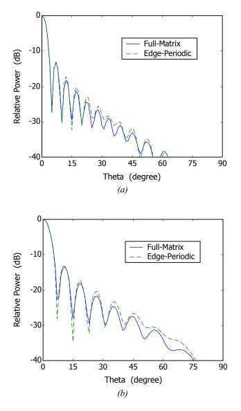
Fig. 6: Co-polarized far-field radiation patterns of a nonuniform 24x24-element array of microstrip dipoles: (a) Eplane, (b) H-plane. Hybrid Edge-Periodic plots are nonoptimal results computed using a total of 7 edge element rings with a 4-ring overlap, while all other array parameters are the same as in Fig. 5.
