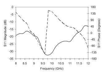
Fig. 11. MoM simulation of  $S_{11}$  for a 2  $\times$  2 one lower slot, one strip, and one upper slot waveguide array. (a) Magnitude (solid line) and (b) phase (dashed line).
