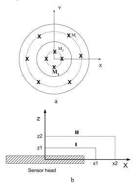
Figure 1. a) Set of dipole sources (X's); the two solid lines are the inner and outer current loop of the GEM-3 sensor. b) Control surface (I) employed to determine dipole sources and the testing surface (II) used for evaluating the accuracy of the field from these sources.
