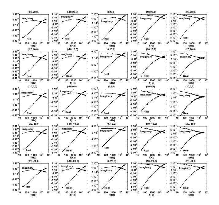
Figure 3 Comparison of SPA (markers) and MAS (lines) values ( $H_z^s$ ) for a prolate spheroid (a=4cm, b=24cm) in a 5x5 grid of sensor locations.  $\sigma = 4 \times 10^6$ ,  $\mu_r = 100$ ,  $x_0 = y_0 = 0$ ,  $z_0 = -30cm$ ,  $\phi_0 = 0$ ,  $\theta_0 = \pi/4$ .
