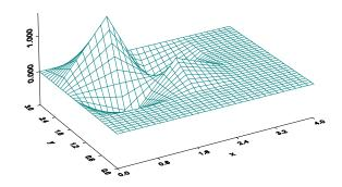
Fig. 11. Linear wavelet-like basis function obtained from a 2nd level x and 2nd level y function.
