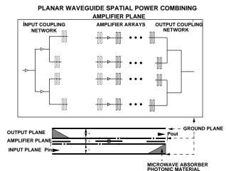
Fig. 2. Aperture-coupled planar waveguide amplifier array.
