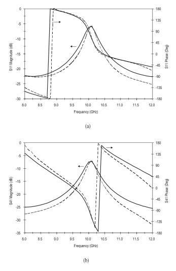
Fig. 7. MoM (solid line) and HFSS (dashed line) comparison of the scattering parameters for one lower slot, two strips, and one upper slot waveguide transition. Magnitude and phase:
