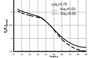
**Fig.3** : Ratio of resonant frequencies of the second to first even modes versus angle  $\alpha$ .
