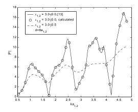
Figure 2. Backscattered field versus electrical size  $ka_{1,2}$  for two dielectric loaded identical semi-circular channels with  $a_{1,2}/b_{1,2}=1.0$  and  $\phi_i=90^o$ .
