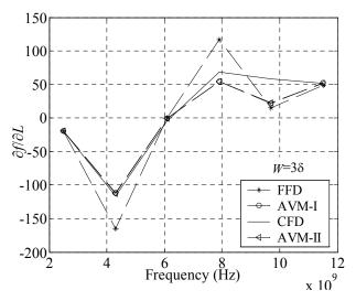
Fig. 9. Derivative of f with respect to L for the printed filter.
