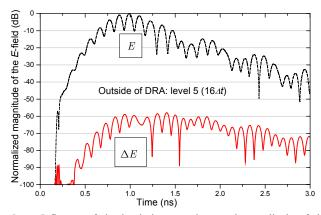
Fig. 5. Influence of the local time stepping on the amplitude of the electric field at a point located outside the DRA. The arbitrarily chosen point is updated with a local time step corresponding to 16 times the fundamental time step. The upper curve (E) shows the E-field magnitude in this point and the lower curve  $(\Delta E)$  the difference between the simulations performed with and without local time stepping.
