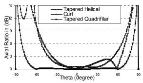
Fig. 8. Computed axial ratio versus the elevation angle.  $\theta$  for the three antennas mounted on infinite ground plane.
