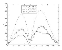
Figure 7. Echo pattern width versus the scattering angle  $\phi$  for two dielectric loaded identical semi-elliptic channels with ka<sub>1,2</sub>=1.5, a<sub>1,2</sub>/b<sub>1,2</sub>=2.0, kd=5.0 and  $\phi_i = 60^{\circ}$ .
