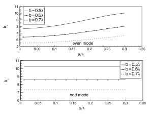
Fig. 4. The second cutoff wavelength versus strip width for even and odd TM modes.
