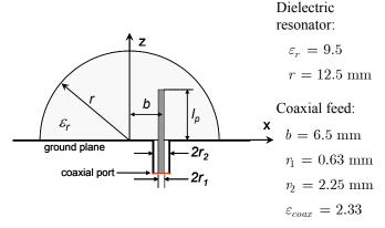
Fig. 2. Schematic cross section of the probe fed hemispherical DRA.
