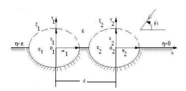
Figure 1. Scattering geometry of two lossy dielectric loaded semi-elliptic channels in a ground plane.
