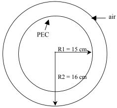
Figure 7. A perfectly conducting sphere.
