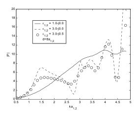
Figure 3. Backscattered field versus electrical size  $ka_{1,2}$  for two dielectric loaded identical semi-elliptic channels with  $a_{1,2}/b_{1,2}=2.0$  and  $\phi_i=90^o$ .
