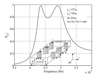
Fig. 2. Insertion loss  $|S_{21}|$  of the filter.
