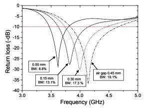
Fig. 12. Return loss of the hemispherical DRA with different air gaps between the dielectric and the ground plane. The figure illustrates the shift of the resonance frequency and the increase of the relative bandwidth when the air gap becomes thicker.
