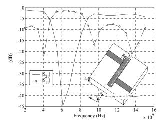
Fig. 7. Reflection and transmission coefficients of the printed filter.
