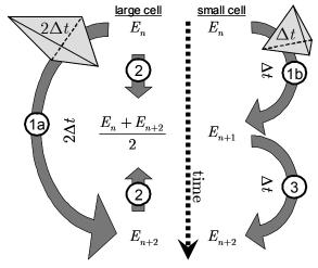
Fig. 1. Principle of application for local time steps at the boundary between sub-domains (two-level system). The chronology is indicated by the encircled numbers. An artificial half-step ② is created in the large cell to obtain data required to perform the update ③.
