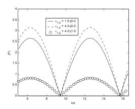
Figure 5. Backscattered field versus electrical separation distance kd for two dielectric loaded identical semi-elliptic channels with ka<sub>1,2</sub>=2.0, a<sub>1,2</sub>/b<sub>1,2</sub>=1.5 and  $\phi_i = 60^{\circ}$ .
