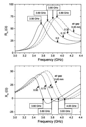
Fig. 11. Effect of an air gap between DRA and ground plane on the input impedance  $Z_{\rm in}$  of the DRA. The rounded probe has a length of 8.0 mm. The  $R_{\rm in}$  (upper graph) and  $X_{\rm in}$  (lower graph) indicate the real and imaginary part of the input impedance respectively.
