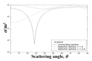
Fig. 10. Normalized bistatic cross-section in the H plane of a partially buried dielectric sphere vs. the scattering angle  $\theta$  for ka = 2.0, d = 0.5a, and  $\varepsilon_r = \infty$ , 4, 2.3.
