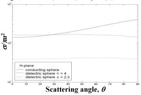
Fig. 6. Normalized bistatic cross-sections in the H plane of a partially buried dielectric sphere vs. the scattering angle  $\theta$  for ka = 1.0, d = 0.5a, and  $\varepsilon_r = \infty$ , 4, 2.3.
