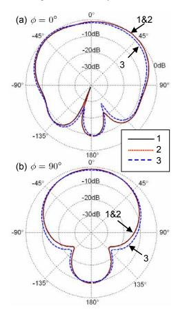
Fig. 13. Radiation patterns of the DRA at 3.6 GHz in two principal planes: (a) plane containing the probe (E-plane), (b) orthogonal plane (H-plane). The patterns are represented for three configurations: (1) 1 mm cut probe, (2) 8 mm rounded probe with 0.3 mm air gap around the probe, (3) 8 mm rounded probe plus air gap between the ground plane and the dielectric.
