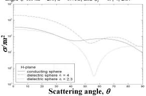
Fig. 8. Normalized bistatic cross-section in the H plane of a partially buried dielectric sphere vs. the scattering angle  $\theta$  for ka = 2.0, d = 0.75a, and  $\varepsilon_r = \infty$ , 4, 2.3.
