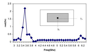
Figure 10. Input impedance of rectangular patch antenna c=100mm, d=76mm, a=25mm, b=19mm, xc=0, yc=0,  $\varepsilon_r$ =2.2.
