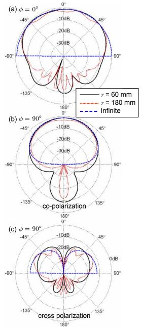
Fig. 14. Radiation patterns near the first resonance (3.6 GHz) for the hemispherical DRA with rounded probe (length 8 mm). The different curves correspond to the given radii r of the circular ground plane. (a) E-plane copolarized pattern  $E_{\theta}$ , (b) H-plane co-polarized pattern  $E_{\phi}$ , (c) H-plane cross-polarized pattern  $E_{\theta}$ . The cross-polarized component in the E-plane is too small to be represented in this scale.
