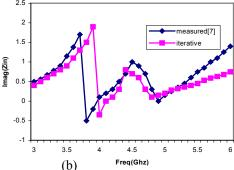
Figure 9. Input impedance of a rectanglar patch antenna as a function of frequency, (a) real part and (b) imaginary part.
