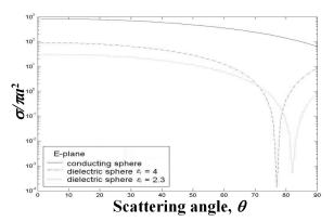
Fig. 5. Normalized bistatic cross-sections in the E plane of a partially buried dielectric sphere vs. the scattering angle  $\theta$  for ka = 1.0, d = 0.5a, and  $\varepsilon_r = \infty$ , 4, 2.3.
