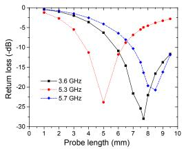
Fig. 7. Return loss as a function of the probe length at three different frequencies.
