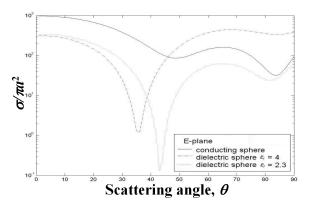
Fig. 7. Normalized bistatic cross-section in the E plane of a partially buried dielectric sphere vs. the scattering angle  $\theta$  for ka = 2.0, d = 0.75a, and  $\varepsilon_r = \infty$ , 4, 2.3.
