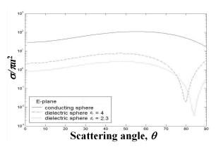
Fig. 3. Normalized bistatic cross-sections in the E plane of a partially buried dielectric sphere vs. the scattering angle  $\theta$  for ka = 1.0, d = a, and  $\varepsilon_r = \infty$ , 4, 2.3.
