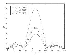
Figure 6. Echo pattern width versus the scattering angle  $\phi$  for two dielectric loaded identical semi-elliptic channels with ka<sub>1,2</sub>=1.5, a<sub>1,2</sub>/b<sub>1,2</sub>=2.0, kd=5.0 and  $\phi_i = 90^{\circ}$ .
