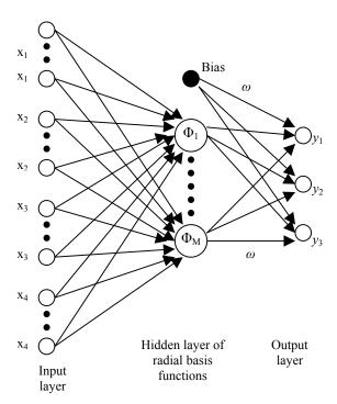
Fig. 2. Radial basis function network.
