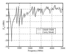
Figure 6. Input impedance comparison using EMAP5-FMM and cavity model.
