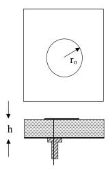
Fig. 1. Geometry of a circular microstrip antenna.
