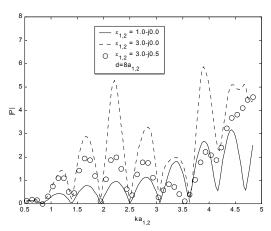
Figure 4. Backscattered field versus electrical size  $ka_{1,2}$  for two dielectric loaded identical semi-elliptic channels with  $a_{1,2}/b_{1,2}=2.0$  and  $\phi_i=45^o$ .
