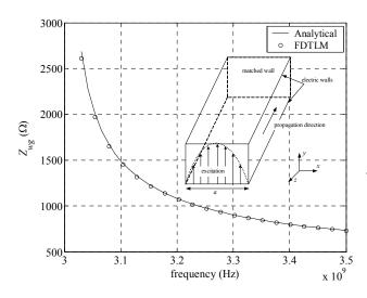
Fig. 10. The wave impedance of the waveguide vs. frequency at a = 5 cm.
