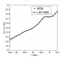
Fig. 3. RCS frequency response of the cylinder.
