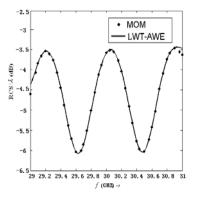
Fig. 5. RCS frequency response of the strip.
