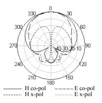
Fig. 19. Simulated radiation pattern of the higher band at 1.786 GHz of the antenna shown in Figure 16, with the dimensions given in the caption of Figure 17.
