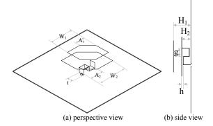
Fig. 21. Geometry of the meandering strip fed stacked patches with truncated corners for circular polarization.
