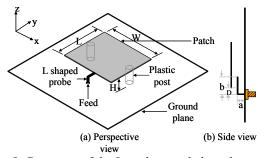
Fig. 5. Geometry of the L-probe coupled patch antenna.
