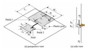
Fig. 16. Geometry of the dual-band patch antenna with combined dual L-probe feed.
