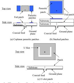
Fig. 3. Three broadband coaxial fed microstrip patch antennas.
