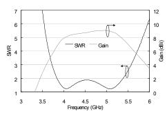
Fig. 7. Simulated SWR and gain versus frequency of the L-probe coupled antenna of Figure 6 with the following dimensions: W=30 mm,L=25 mm,H=6.6 mm, a=5.5 mm, b=10.5 mm, d=2 mm.
