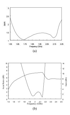
Fig. 22. (a) Simulated SWR (b) simulated AR and gain of the antenna shown in Figure 21 with the following dimensions:  $W_1=56 \text{ mm} (0.378\lambda_0)$ ,  $W_2=66 \text{ mm} (0.445\lambda_0)$ ,  $A_1=17 \text{ mm} (0.115\lambda_0)$ ,  $A_2=23.5 \text{ mm} (0.159\lambda_0)$ ,  $H_1=18.5 \text{ mm} (0.125\lambda_0)$ ,  $H_2=11.5 \text{ mm} (0.078\lambda_0)$ , t=16mm  $(0.108\lambda_0)$ ,  $g=1.45 \text{ mm} (0.01\lambda_0)$ , h=9.3mm $(0.063\lambda_0)$ .
