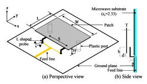
Fig. 9. Geometry of the twin-L-probe fed patch antenna.
