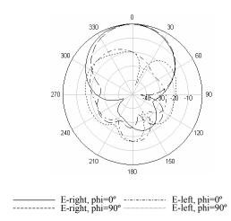
Fig. 23. Simulated radiation pattern of the higher band at 2.036 GHz of the antenna shown in Figure 21, with the dimensions given in the caption of Figure 22.
