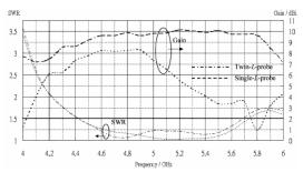
Fig. 10. Measured SWR and gain of the twin-L-probe coupled patch of Figure 9 with the following dimensions: L=22 (0.367 $\lambda$ ), H=6 (0.1 $\lambda$ ), W=44 (0.733 $\lambda$ ), T=0.3 (0.005 $\lambda$ ), a=4.5 (0.075 $\lambda$ ), b=12 (0.2 $\lambda$ ), v=2(0.033 $\lambda$ ), d=0(0 $\lambda$ ), s=28.6(0.477 $\lambda$ ). The case of single L-probe coupled patch is also shown for comparison. (From Mak et. al. [9], c 2005 IEEE)
