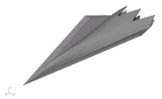
Fig. 7. Geometrical model of FLAMME aircraft.
