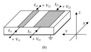
Fig. 1. The considered interconnect: (a) cross-section view; (b) adopted references for terminal voltages and currents.
