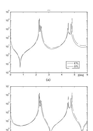
Fig. 8. Near-end (a) and far-end (b) crosstalk voltage normalized to the input voltage, Case 2.
