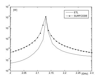
Fig. 5. Absorbed power for ideal dielectric, Case 1.
