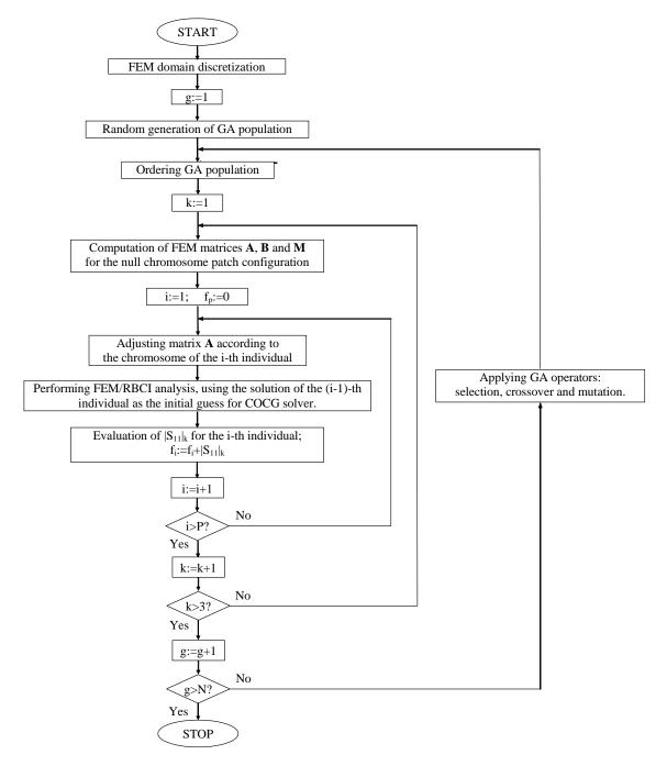
Fig. 3. A flowchart of the whole optimization procedure.
