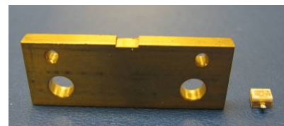
Fig. 15. The CREE transistor sits on this block.
