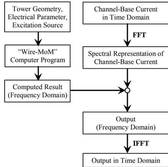
Fig. 2. Time domain transient analysis using Wire-MoM.
