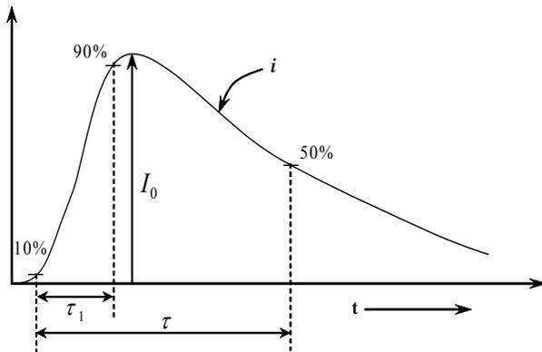
Fig. 1. Waveform of Heidler’s model of current source.
