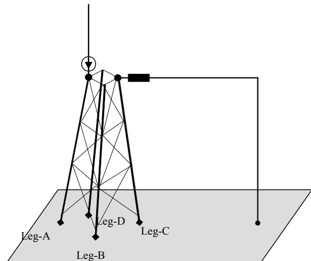
Fig. 5. Computation of current and surge response of 42m high GSM tower.
