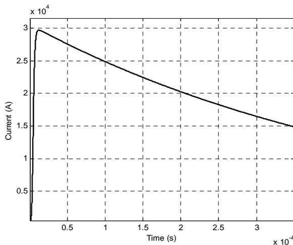
Fig. 3. Waveshape of Heidler's model of current source.
