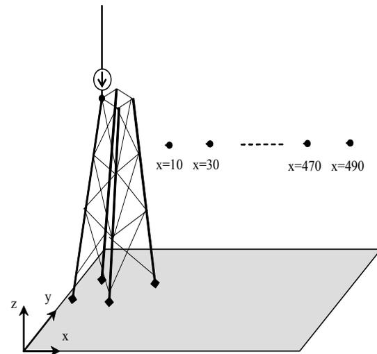
Fig. 11. Near field points for field computation.
